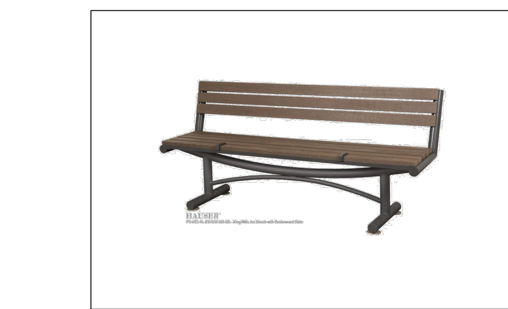
5 BENCH NTS MODEL: P.S 682-AL-EK-EK-SP-BD-T4 MANUFACTURER: HAUSER SITE FURNITURE (800-268-1528 -TRUDY WALKER) PRODUCT: KINGS HILL ARC BENCH WITH ENVIRO WOOD SLATS SIZE: 188.0cm X 56.5cm X 74.4cm SEAT HEIGHT: 45.1cm COLOUR: WALNUT OTHER: GUNMETAL POWDER COAT FINISH NOTE: OPTIONAL SKATEBOARD DEFLECTOR OR APPROVED EQUAL
