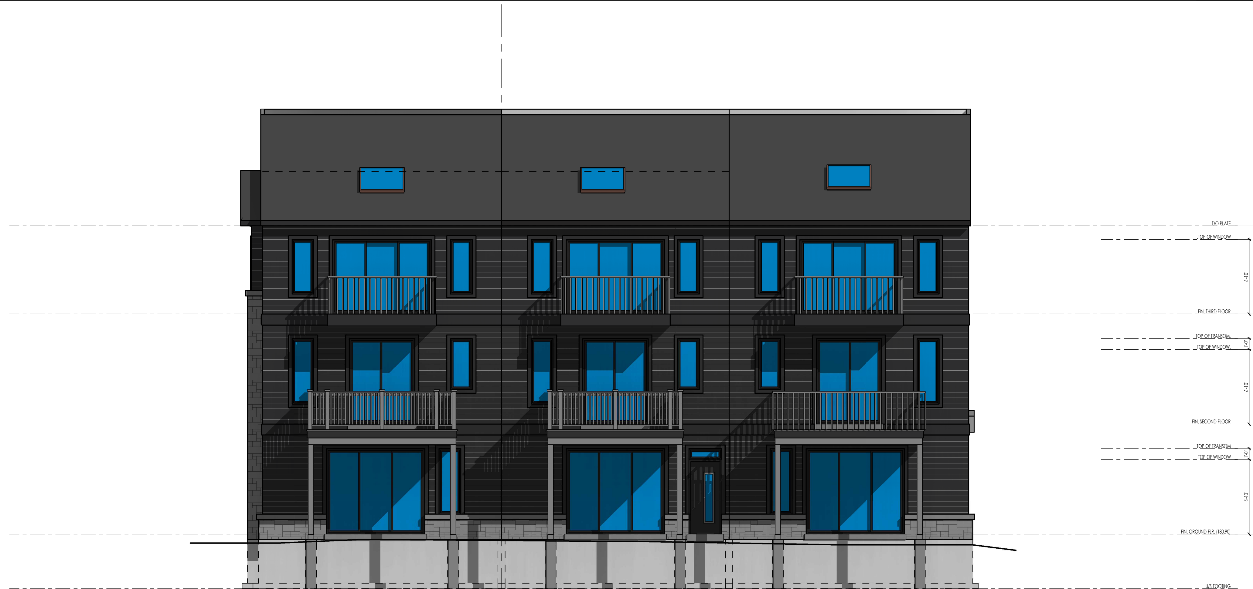
① BLOCK 5 - REAR ELEVATION 3/16" = 1'-0"
