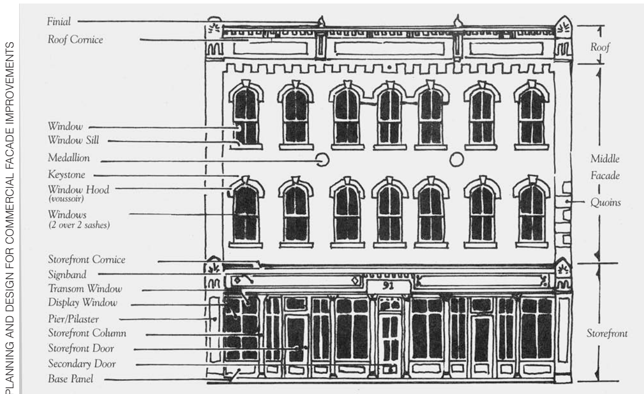
Components of a Commercial Building
