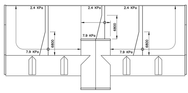
**KEY PLAN (SNOW BUILD UP ON FLAT ROOF)**
