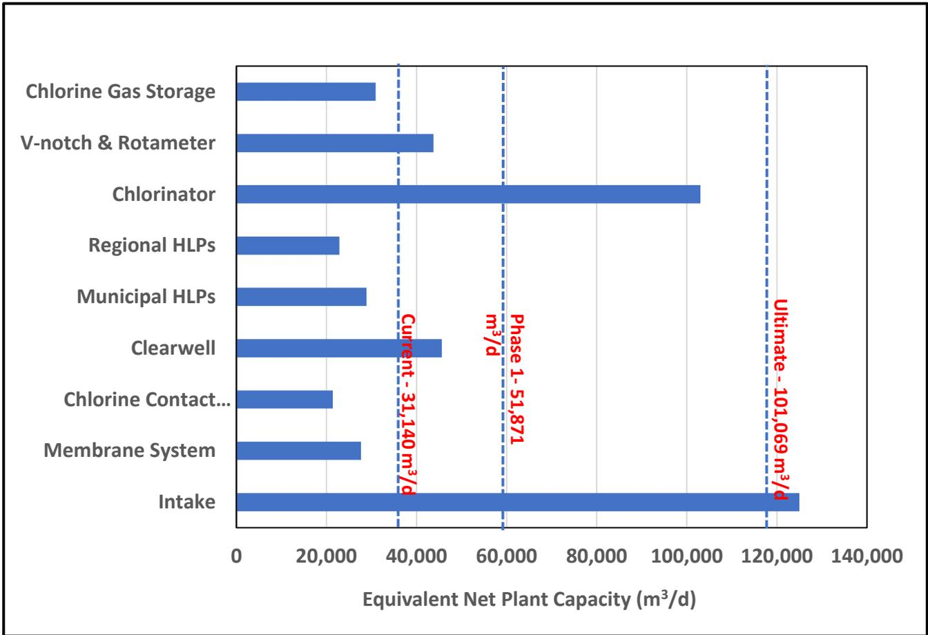
Figure 2 Equivalent Net Plant Capacity of Unit Processes
