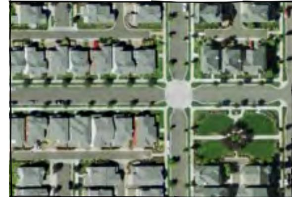
Pedestrian access and safety is improved in this location with: a. the use of curb extensions to reduce crossing distances and traffic speeds; b. sidewalks; and, c. a pedestrian scramble at the main park entrance. Source: Google
