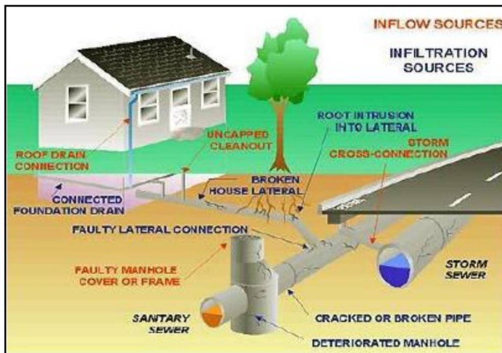
Figure 10-1 Inflow and Infiltration Sources
